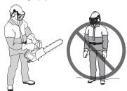
Always hold the saw with both hands. The right hand should be on the top handle, and the left hand on the front handle. All people, whether right or left handed, should use this grip. Use a firm grip with thumbs and fingers encircling the chain saw handles.
