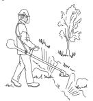
5 Keep a good balance and a firm foothold. Do not overreach. Keep proper footing and balance at all times. 6 Always hold the machine with both hands. Hold the machine on the right side of your body. Keep all parts of your body away from the hot surfaces. Keep all parts of your body away from the rotating cutting attachment.
