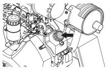
• Check the engine's oil level, see instructions under heading "Daily maintenance".
