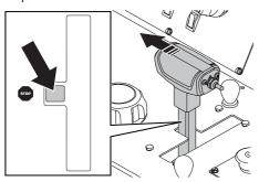
1 Start the engine, turn the Engine start switch to ignition on position. Follow the procedure in the engine manual.
