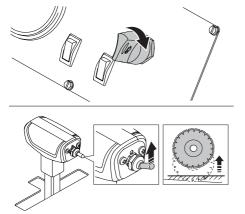
Put Forward/Reverse control lever into the Stop/Neutral position.
