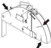
• Never use a broken or damaged blade guard.
