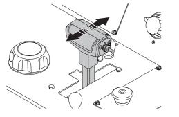
WARNING! Do not put transmission in neutral while the machine is parked on a grade or hill. The operator will lose control and injury or damage could occur.
