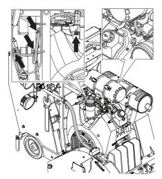
• Look for leakage on fuel and hydraulics system. Tighten or replace as necessary.
