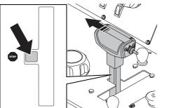
• Raise the diamond blade out of the cut by pressing the Raise/lower switch on the control lever upward until the diamond blade clears the surfaces.
