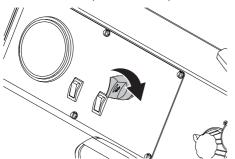
Push the Forward/Reverse control lever forward for forward saw movement, or to the rear for reverse saw movement.
