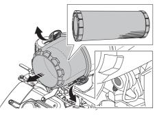
• Clean the filter by blowing the element from inside out.
