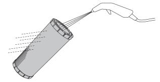
Replace any damaged filters or gaskets and check air hose and clamps for damages or looseness. Tighten or replace as required.
