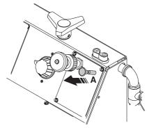
• Turn the Engine start switch to the engines start position until the engine starts, then release the switch. It will return to ignition on position automatically. If the engine does not start, repeat these steps.
