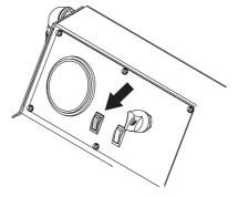
• Put the Forward/Reverse control lever into the Stop/ Neutral position. The engine will not start unless the lever is in the Stop/Neutral position.
