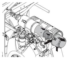
CAUTION! The 2 air filter housing clamps can not be closed unless the outer air filter is properly installed.
