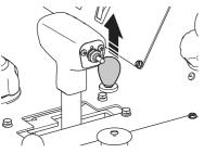
• The saw can now be moved by standing behind it and pushing (while holding the handlebars).
