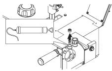
• Refill the reservoir with new oil. Ensure that machine is level prior refilling.
